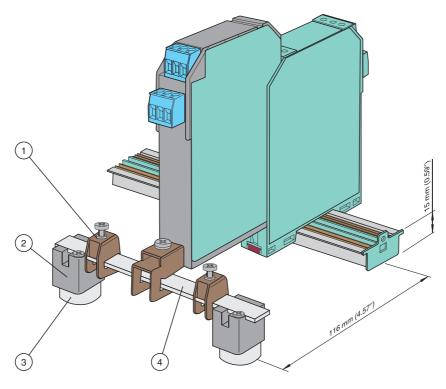
Keep the drilling distance of 116 mm between center mounting rail and center grounding bar.
