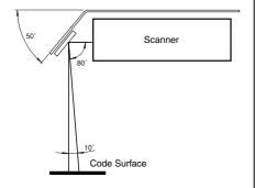
The deviation mirror is attached to the scanner with 4 screws, which are supplied in the delivery package.
