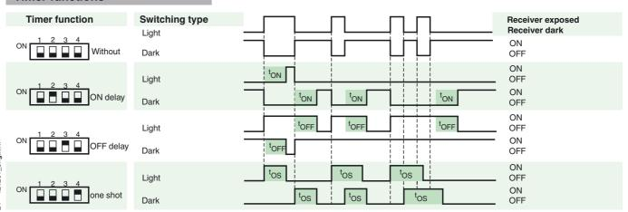
Time  $t_{\mbox{\scriptsize ON}}, t_{\mbox{\scriptsize OFF}}$  and  $t_{\mbox{\scriptsize OS}}$  are adjustable from 0.02 to 1 seconds. The Light-/Dark-Switch (Left, outer switch) is shown in the "Dark ON" position.
