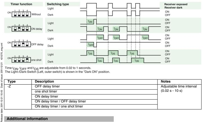
Time  $t_{\mbox{\scriptsize ON}}, t_{\mbox{\scriptsize OFF}}$  and  $t_{\mbox{\scriptsize OS}}$  are adjustable from 0.02 to 1 seconds.
