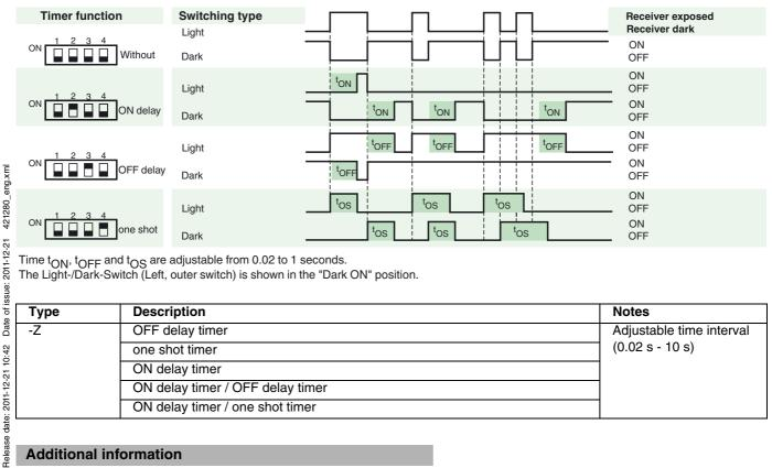
Time  $t_{ON}$ ,  $t_{OFF}$  and  $t_{OS}$  are adjustable from 0.02 to 1 seconds. The Light-/Dark-Switch (Left, outer switch) is shown in the "Dark ON" position.
