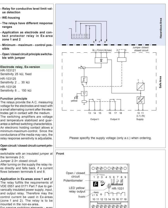
For passive switching elements - even those without approval - may the relay be used as contact protector relay. An additional approval is not required.
